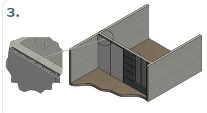
As a last step, plaster wallboards or particle boards are fixed on the slat framework with screws.
